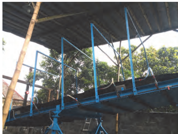
Photo 1. The tilted plot and the 5-sprinklers rainfall simulator (phot. L. Sedyowati)
