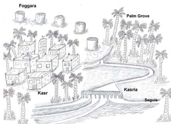
Fig. 2. Simplified diagram of a foggara; source: own elaboration
