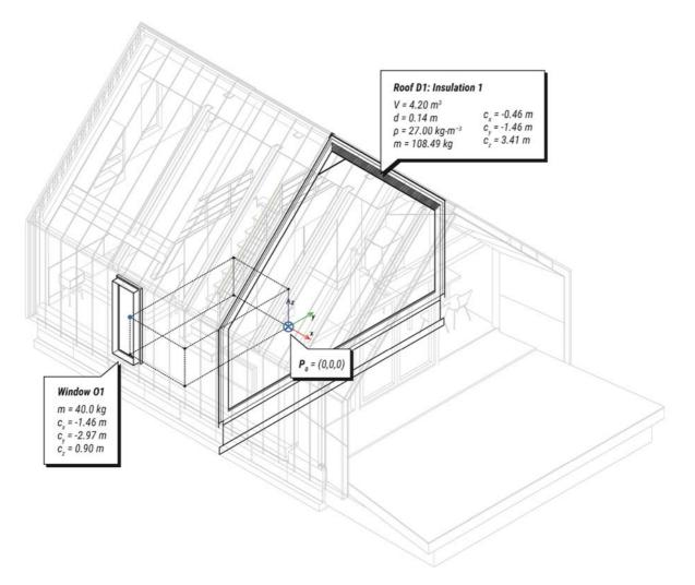
Fig. 3. Axonometric scheme of the geometry analysis; V = volume, d = layer thickness,  $\rho =$  material density, m = mass, c = center of mass, Po = model origin; source: own elaboration
