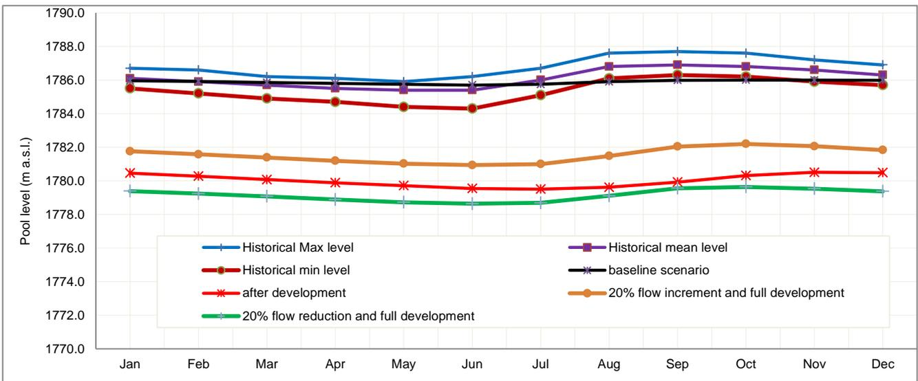
Fig. 8. Simulation results of pool level (m a.s.l.) in Lake Tana for different flow and development scenarios; source: own study
