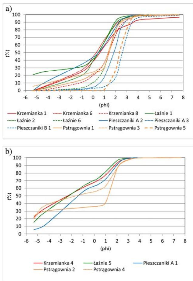
Fig. 5. Grain size distribution curves of the deposits of the selected spring-head alcoves in Knyszyńska Primeval Forest: a) aquifer deposits, b) bottom deposits; source: own study
