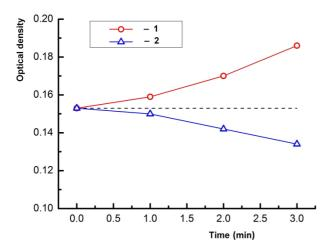
Fig. 2. Dependences of the optical density of the suspension near the electrodes from the time of electric current action with current density of  $0.008 \text{ A} \cdot \text{cm}^{-2}$ : 1 = anode; 2 = cathode; the dashed line means the initial value of the optical density of the suspension; source: own study
