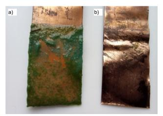
Photo 1. Electrodes after the action of electric current on the suspension: a) anode, b) cathode (phot. *I. Bordun*)
