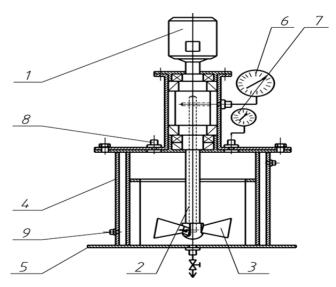
Fig. 1. Scheme of the laboratory-experimental installation: *I* = electric motor, 2 = shaft, 3 = cavitational device, 4 = tank,
