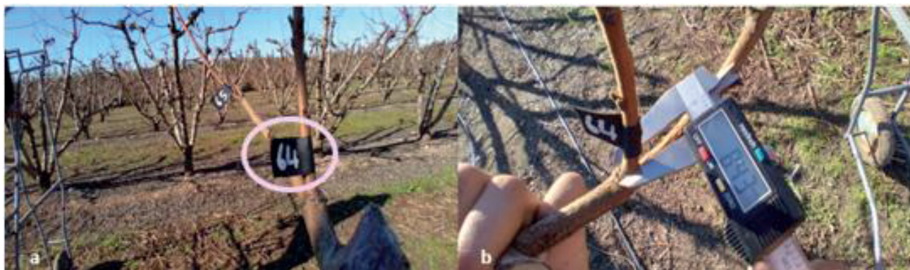
Photo 1. Mixed branches: a) labelled, b) diameter measurement with digital calliper (phot.: A. Zegoumou)
