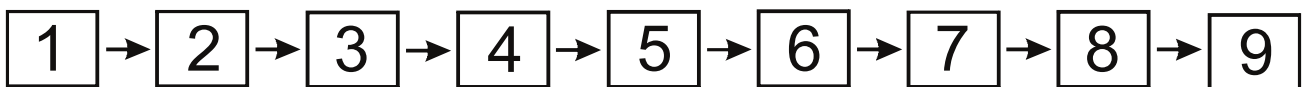
Fig. 2. Flowchart of the investigations and statistical analyses performed for the pipe aerator with steel Bialecki rings of 12 mm and 25 mm diameter: 1 = construction of the measuring rig, 2 = methodological development of the investigations, 3 = measurements, 4 = estimation of a measurement uncertainty, 5 = statistical analysis of measurements, 6 = determination of formulas for calculations oxygen content in water leaving the aerator, 7 = a statistical analysis for a verification of the correctness of the fitting of the logarithmic model for calculating the content of the oxygen dissolved in water leaving the aerator, 8 = development of a nomogram for reading the air flow rate related to the required content of the oxygen O_2 dissolved in the water leaving the aerator, 9 = determination of the energy efficiency coefficient for the investigated aerator; source: own elaboration
