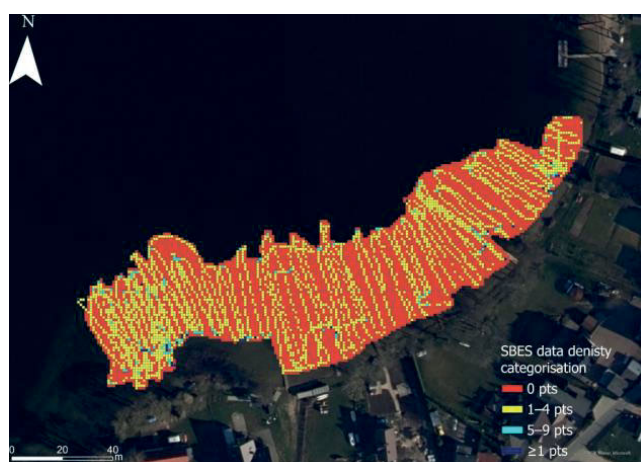
Fig. 5. Singlebeam echosounders (SBES) data density categorisation in a 1×1 m grid for Lake Kłodno; source: own study
