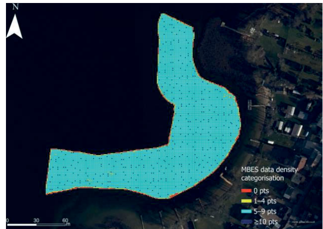
Fig. 9. Multibeam echosounders (MBES) data density categorisation in a 1×1 m grid for Lake Kłodno; source: own study
