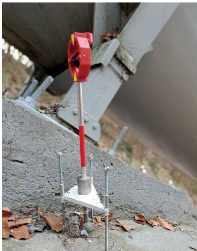
Photo 1. Special mobile geodetic mark (phot.: I. Sidorov)
