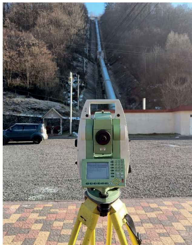
Photo 2. Determination of the heights of reference marks by the method of trigonometric levelling (phot.: I. Sidorov)
