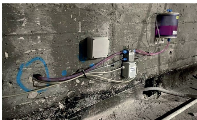
Photo 1. An example of a system used in hydrostatic levelling is the H-Level solution from Sisgeo; source: https://www.geo-instruments.pl/en/projects/monitoring-building-69-wolska-street
