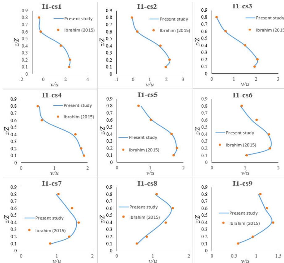
**Fig. 3.** Velocity distribution at selected sections for geometric design (I); I1-cs1–I1-cs9: I1 = usage of the hydraulic variables of test number one (1) on geometry (I) of basin, cs1–cs9 = chosen sections from one (1) to nine (9), location of sections is shown in Fig. 2,  $z/Z$  = certain depth/water depth,  $v/u$  = velocity at certain depth/average velocity; source: own elaboration based on present study and Ibrahim (2015)
