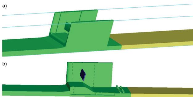
**Fig. 6.** Models of the alternative stilling basin designs: a) alternative design 4, b) alternative design 5; source: own study
