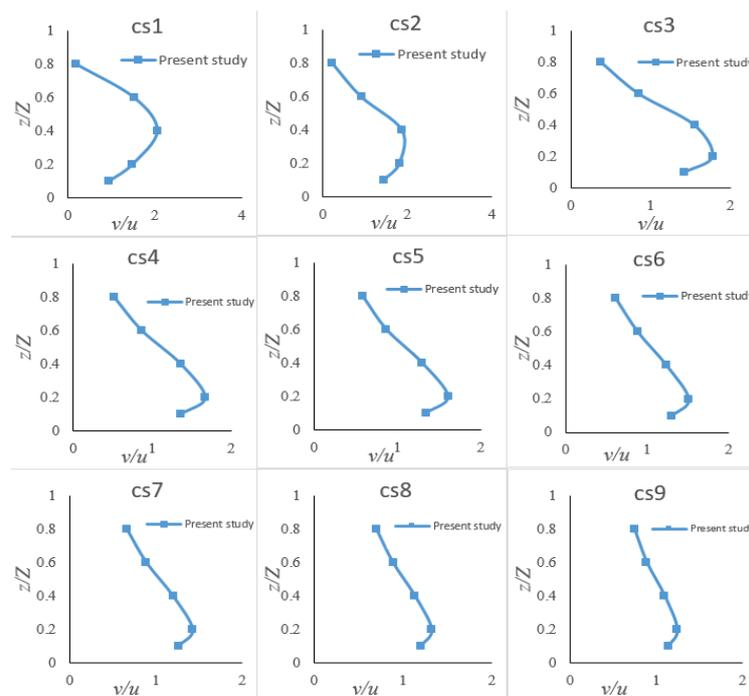
**Fig. 7.** Velocity profile for alternative design 4 – test No. 1; cs1–cs9 = chosen sections from 1 to 9, as in Fig. 2,  $z/Z$ ,  $v/u$  as in Fig. 3; source: own study
