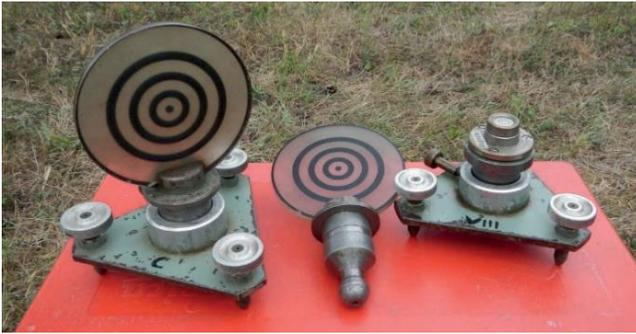
**Photo 1.** Targets for observing the crest displacement using the baseline method (phot.: J. Zaczek-Peplinska)
