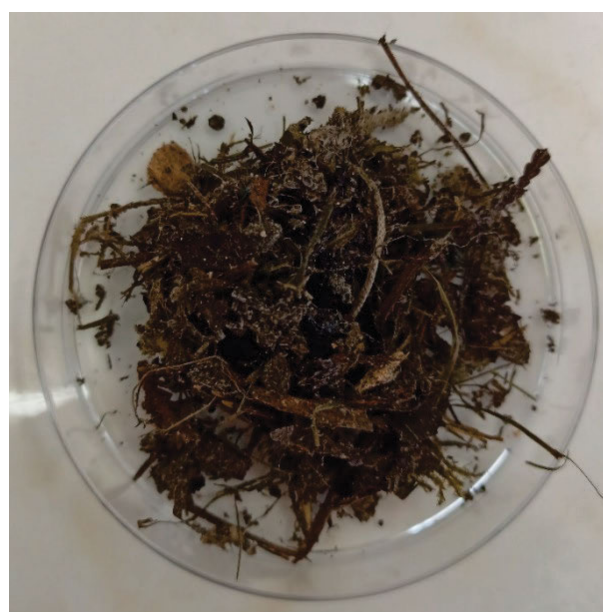
Photo 1. Sample of municipal waste used in the experiment (phot. K. Wolny-Koładka)
