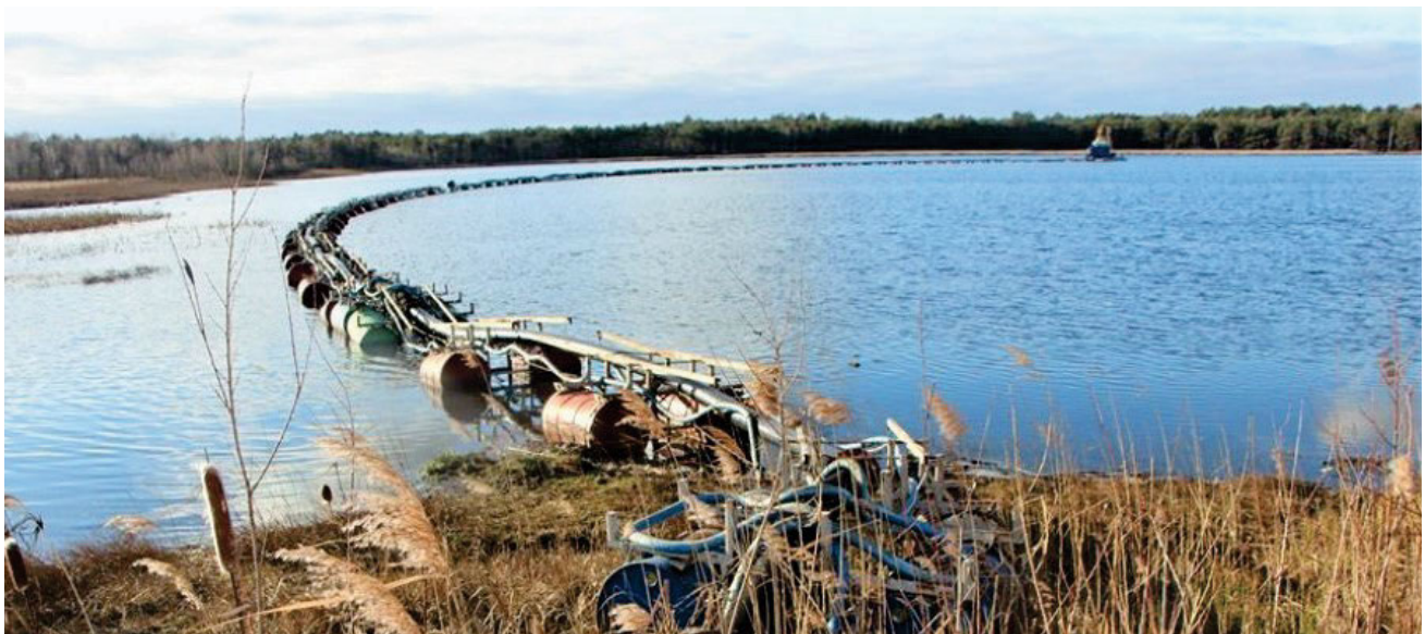
Photo 1. Hydromechanised sapropel extraction from the field on Lake Prybych (Shatsk Lakes, Volyn Region, Ukraine) (phot.: M. Pasichnyk)
