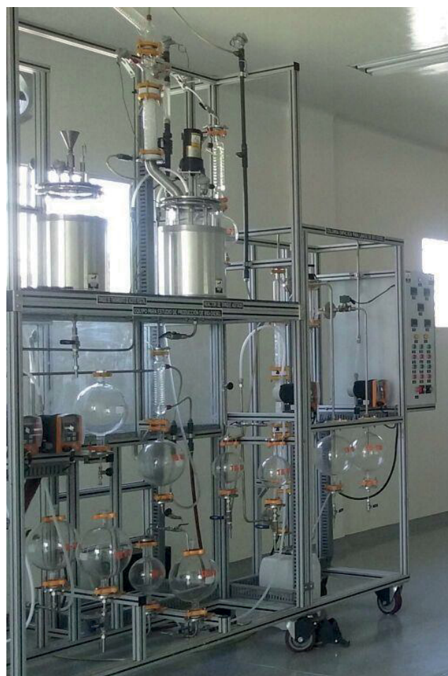
Photo 1. Pilot plant to obtain biodiesel UFPS (phot. N.A. Urbina-Suarez)
